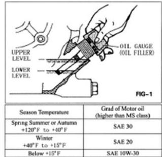
1-5. Remove the oil plug in the vibrator assembly and check the oil level. Make sure the compactor is level when checking. The oil level should be up to the oil plug. Every month or every 200 hours of operation, replace the oil.
