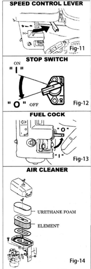
2. Wash the element in kerosene or diesel fuel. Saturate it in a mixture of 3 parts kerosene or diesel fuel and 1 part engine oil. Shake off excessive oil and reinstall.
